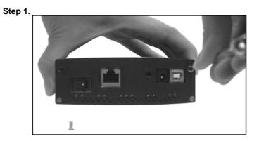
Remove two retaining screws on the rear panel securing the **Rear Panel** and **Body Case (Body Case including Body Outer Cover and Inner Cradle with PCB and Front Cover)**.
